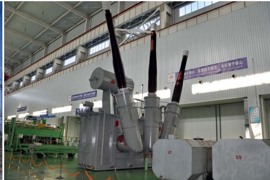
400kV transformer for Venezuela Substation
