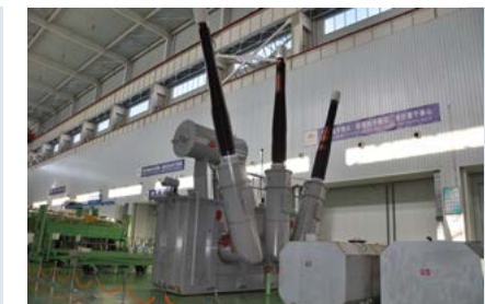
400kV transformer for Venezuela Substation
